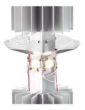
The T1 optical system simulates a pointed light source by utilizing highly efficient multi point Chip On Board (COB) LED emiters, reflectors, and precision external optics. It has high lumen output and impressive optical efficiency.
